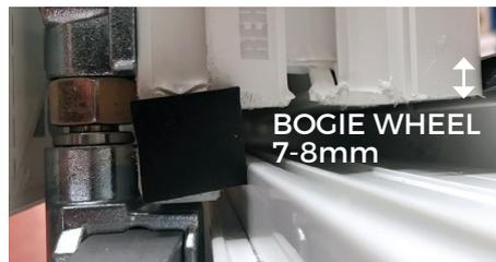
3: The door overlap is to be set at between 7-8mm
