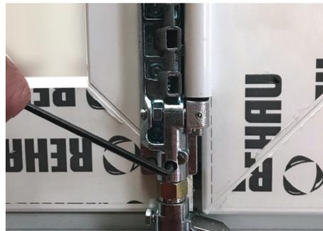
1: Slacken grub screw with 4mm allen key
